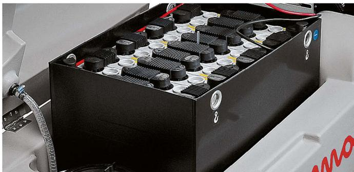
The battery compartment is positioned at the centre of the machine and it is integrated in the tank's volume. All around the batteries, the plastic materials are resistant to oxidising vapours so that any ugly and harmful rust formation is prevented.
