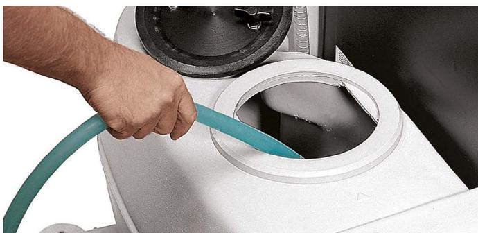
The solution and recovery tanks, in rotational polyethylene, are very strong and are both shock and rust resistant. The solution tank is positioned in the upper part of the machine so that effective and constant water flow onto the brushes is ensured. It is filled through a large opening and it has a holding capacity of respectively 75 litres for Omnia 26 BT and 105 litres for Omnia 32 BT.
